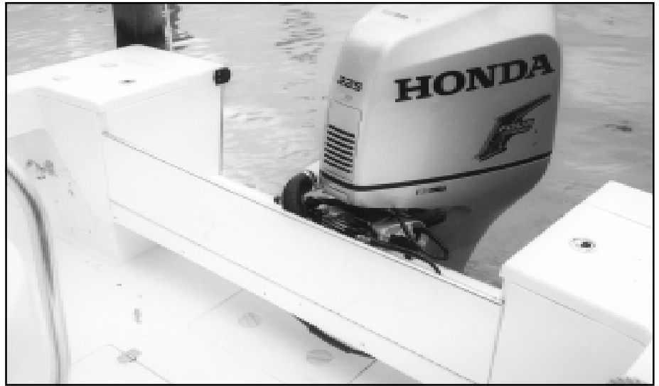
Above: The SeaCraft 23's piano-hinged transom board keeps out green water but still allows for toekick space. The board is long (55") but seemed strong and stiff. It can be folded down to free space so the outboard can be fully trimmed.
